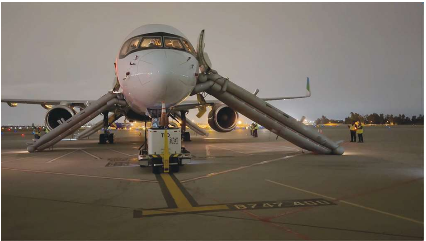
Northern Pacific Airways has successfully completed its mini-evacuation drill for the FAA. The cabin crew opened the doors in 7.04 sec., and slides fully deployed in 12 sec. Credit: Northern Pacific Airways
